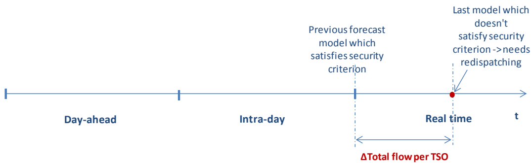
Figure 44. Illustration for real time redispatching case
